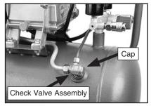
Figure 19. Check valve assembly.
